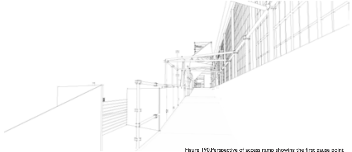
Figure 190. Perspective of access ramp showing the first pause point
