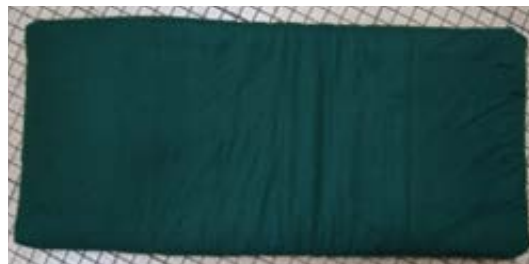
Figure 265. Sheets of cardboard was cut according to the chair profile and stacked next to each other inside the chair to create a seating surface. A 450 x 1000 mm rubber mat is woven from 40mm wide strips of the inner tube of a vehicle tyre. A 400 x 950 x 40 mm piece of foam is covered with a felt cover that can be removed and washed. The covered foam is attached to the rubber mat by pressed-it clips. The 'pillow' is then placed onto the seating surface of the chair to increase comfort & acoustic absorption. The pillow itself can also be used as temporary movable seating with the rubber mat as durable substrate providing a non-slip grip (Author,2010).
