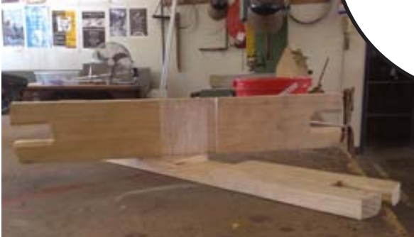
Figure 263. Two 38x114mm pieces of timber are cut to 600mm lengths. The ends are rounded and a slot is cut in each end for a casters to fit through. The two pieces are fixed together with a shiplap joint and secured with wood-glue and wood-screws .A caster is placed in each slot and fixed to the wood with wood-screws. Matching holes are cut in the base of the drum to accommodate the casters. The assembly is placed in the bottom of the drum (Author,2010).
