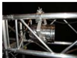
Figure 208. Floodlight temporarily attached to Z-Line truss (Author, 2010).
