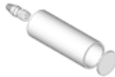
Lit lettering created by fixing a compact fluorescent lamp inside selected tubes. The open ends of the tube are covered with a disc of white translucent acrylic sheet cut to size. Different coloured lamps will provide additional possibilities.
