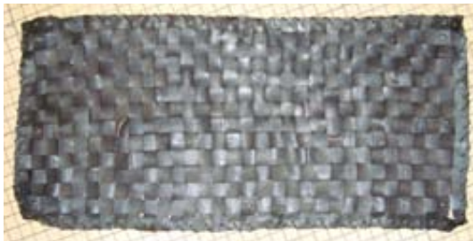
Figure 265. Sheets of cardboard was cut according to the chair profile and stacked next to each other inside the chair to create a seating surface. A 450 x 1000 mm rubber mat is woven from 40mm wide strips of the inner tube of a vehicle tyre. A 400 x 950 x 40 mm piece of foam is covered with a felt cover that can be removed and washed. The covered foam is attached to the rubber mat by pressed-it clips. The 'pillow' is then placed onto the seating surface of the chair to increase comfort & acoustic absorption. The pillow itself can also be used as temporary movable seating with the rubber mat as durable substrate providing a non-slip grip (Author,2010).
