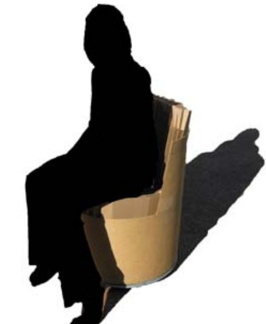
Figure 265. Sheets of cardboard was cut according to the chair profile and stacked next to each other inside the chair to create a seating surface. A 450 x 1000 mm rubber mat is woven from 40mm wide strips of the inner tube of a vehicle tyre. A 400 x 950 x 40 mm piece of foam is covered with a felt cover that can be removed and washed. The covered foam is attached to the rubber mat by pressed-it clips. The 'pillow' is then placed onto the seating surface of the chair to increase comfort & acoustic absorption. The pillow itself can also be used as temporary movable seating with the rubber mat as durable substrate providing a non-slip grip (Author,2010).
