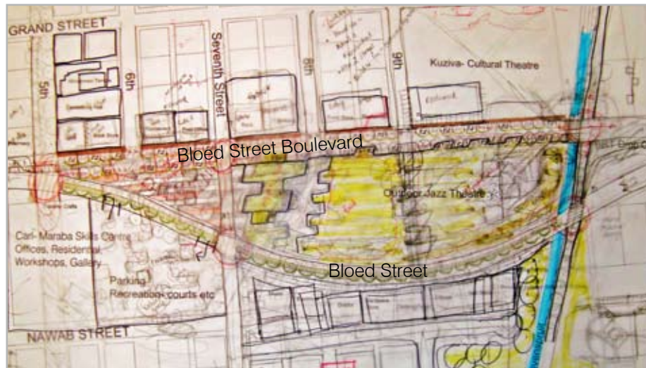
Figure 72. Integrating site with surrounding proposed functions as well as proposing urban design functions along boulevard and calming traffic in Bloed Street (Author, 2009)
