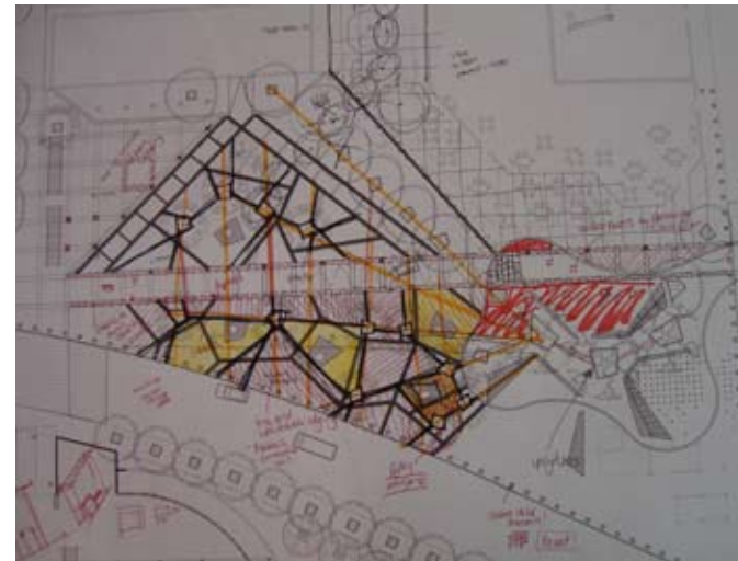
Irregular concrete paving versus grid formation
