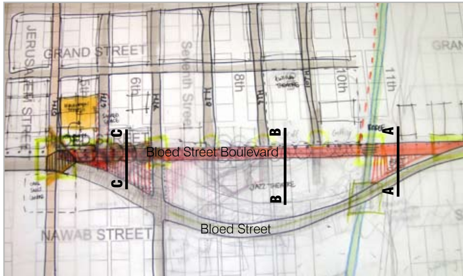
Figure 71. Development of master plan with connections from BRT drop to 5th Street pedestrian spine by proposing pedestrian boulevard along historic route of Bloed Street (Author, 2009)
