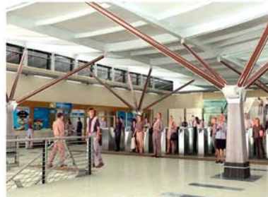
polished black granite skirting tiles, painted grey, steelwork painted white
