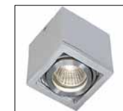
Trebant 230V adjustable, surface mounted light with 50W GU10 halogen lamp, fitted flush with ceiling surface. Two timber ceiling slats to either side of light fittings remain removable for maintenance.
