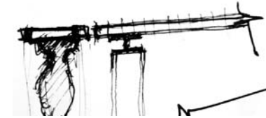
Figure 8.33 Conceptual detail of extension of stage floor area over orchestra pit
