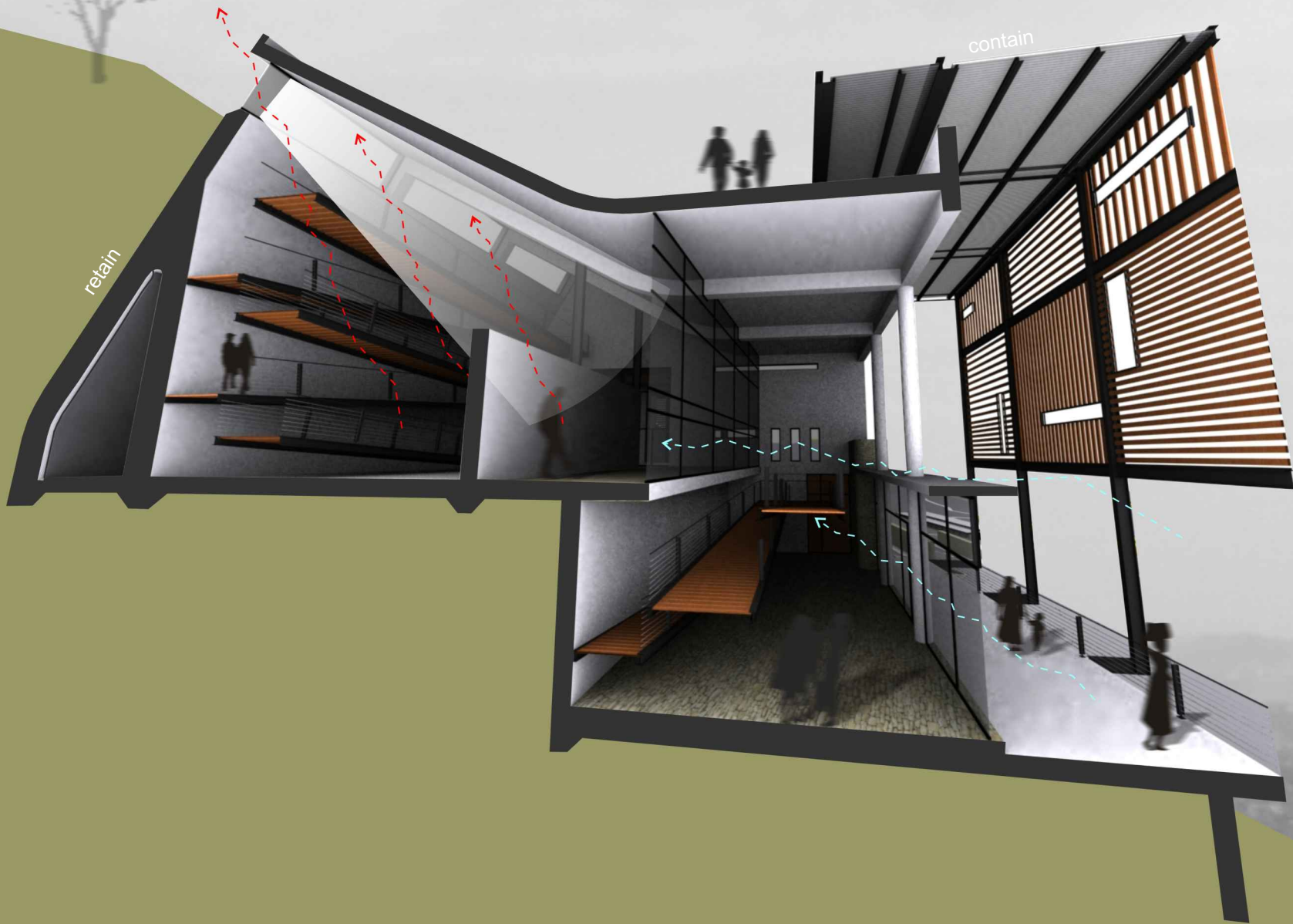
fig. 6.15. Section through visitors centre indicating possible thermal activity. (2010)
