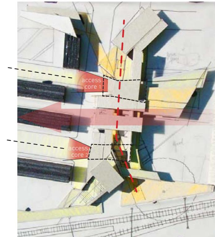
The two access cores line up with the pathways formed by the existing warehouses. These cores are connected to a network of elevated walkways within the structure.
