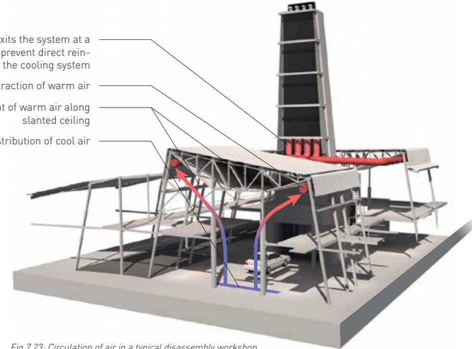
Fig 7.23: Circulation of air in a typical disassembly workshop, Illustrated by Author 2011
