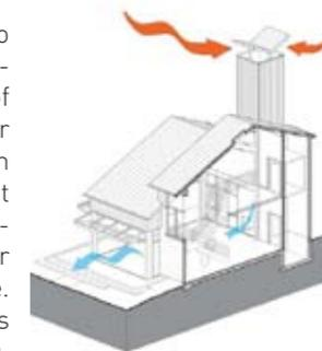
Fig 5.30: Cooling tower's ventilation diagram [Carboun 2010]
