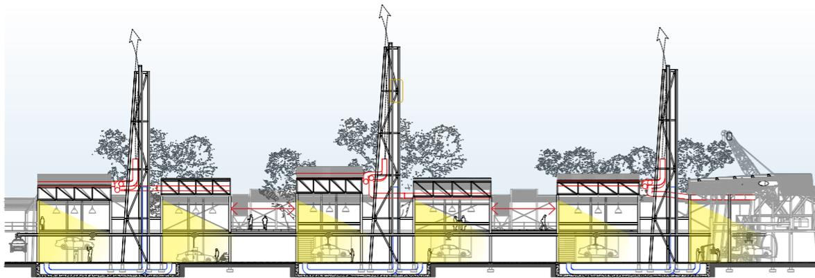
Fig 7.29: Penetration of daylight into the disassembly workshops, Illustrated by Author 2011
