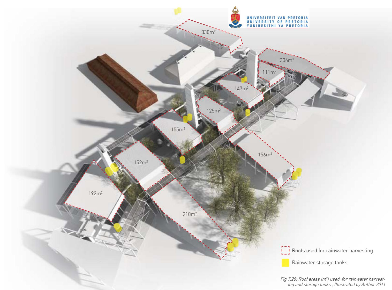
Fig 7.28: Roof areas (m<sup>2</sup>) used for rainwater harvesting and storage tanks, Illustrated by Author 2011
