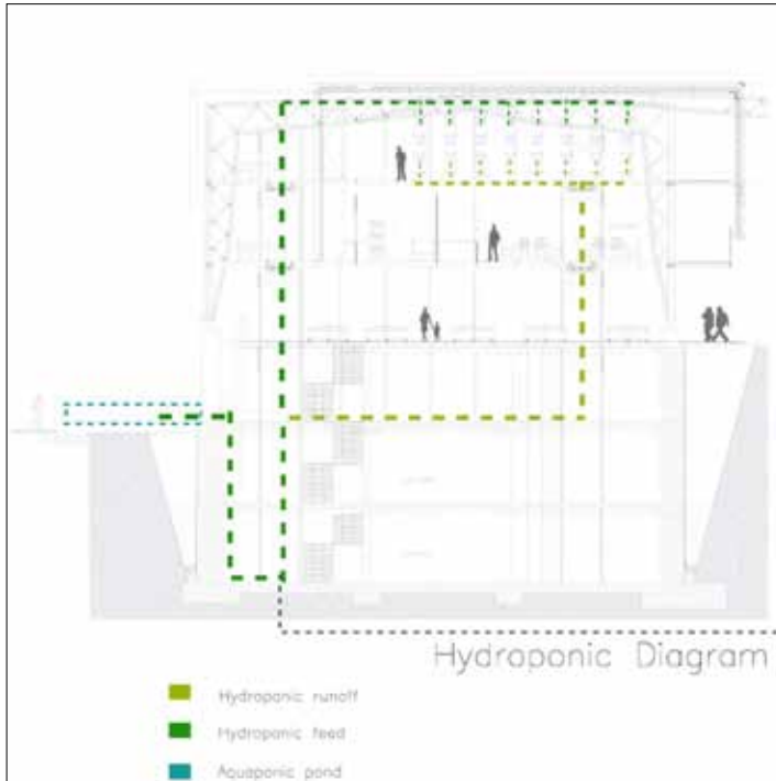
>>111: Hydroponic water circulation diagram.
