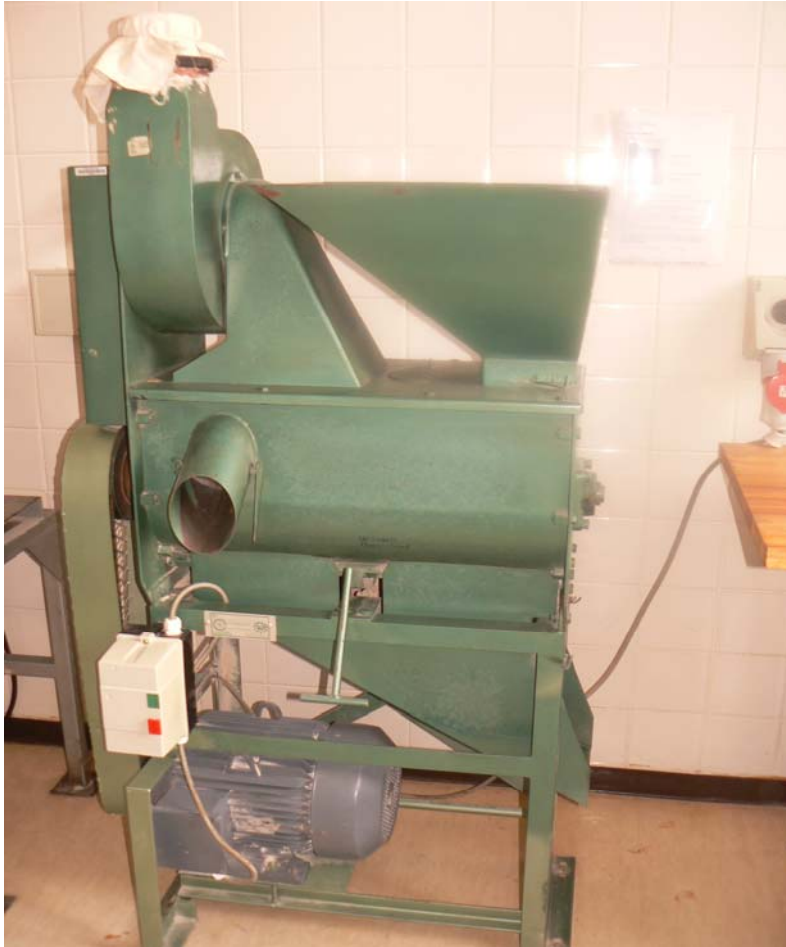
Figure 1.2.6 Prairie Research Laboratory (PRL) type dehuller (Rural Industries Innovation Centre, Kanye, Botswana).
