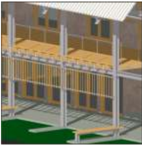
Figure 8.68: Perspective of west facade of training and therapy center indicating timber and steel composite seat and louver system and timber balcony.
