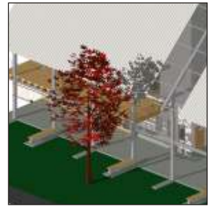
Figure 8.66: Deciduous trees shade the building and garden in summer
