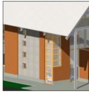
Figure 8.70: South-west elevation of training and therapy center indicating the use of brick, off-shutter concrete and steel for the structural frame and roof.
