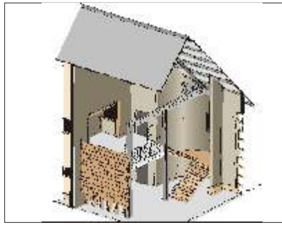
Figure 8.35: The articulation is not based on joining elements, but on maintaining a relationship between components. The lobby of the training and therapy center is a defined space, with the timber screen and steel columns giving definition. The stair, however, is placed in a brick box that suggest continuity with the enclosed structure as in the historic Edwardian tradition.
