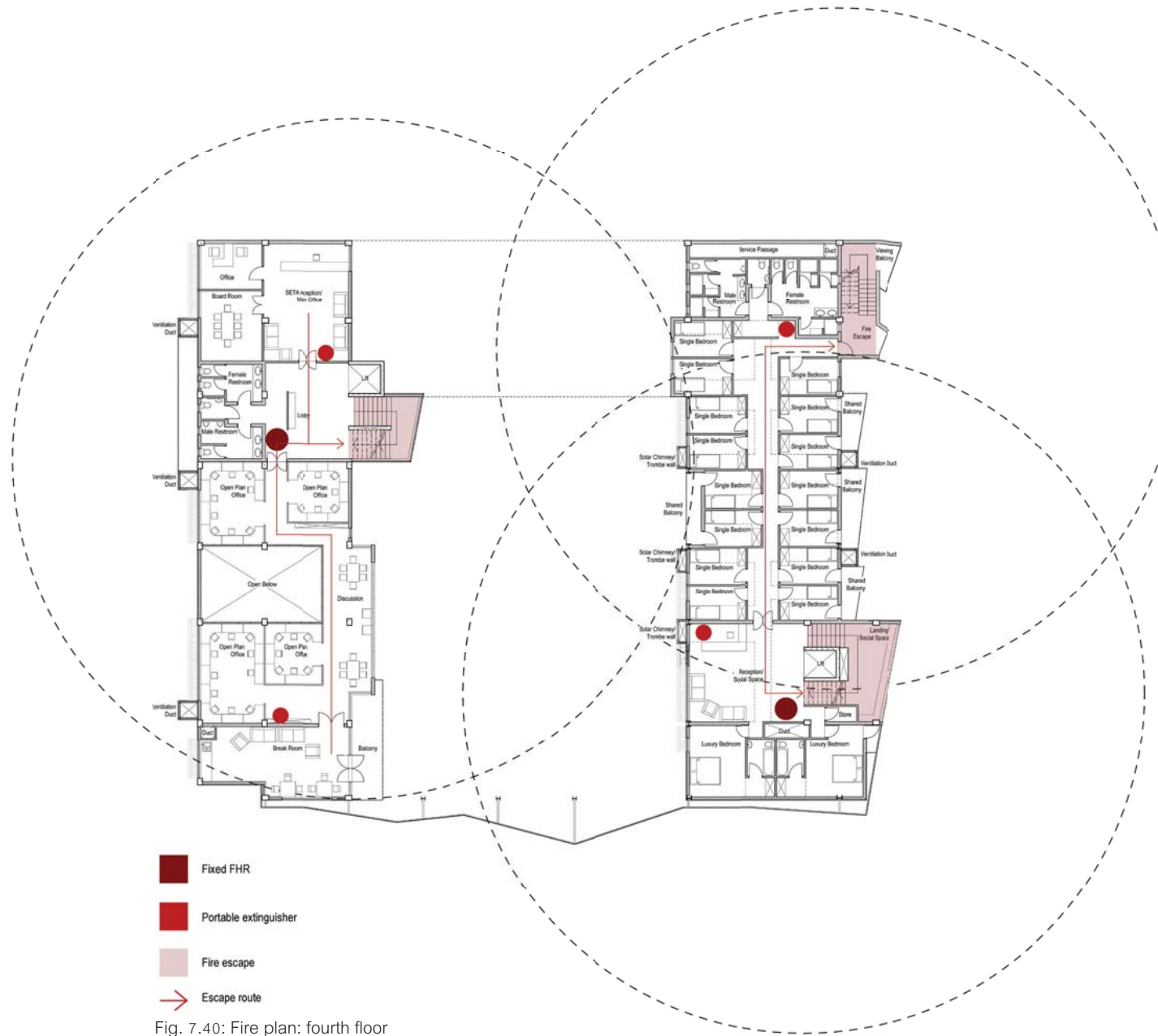
Fig. 7.40: Fire plan: fourth floor
