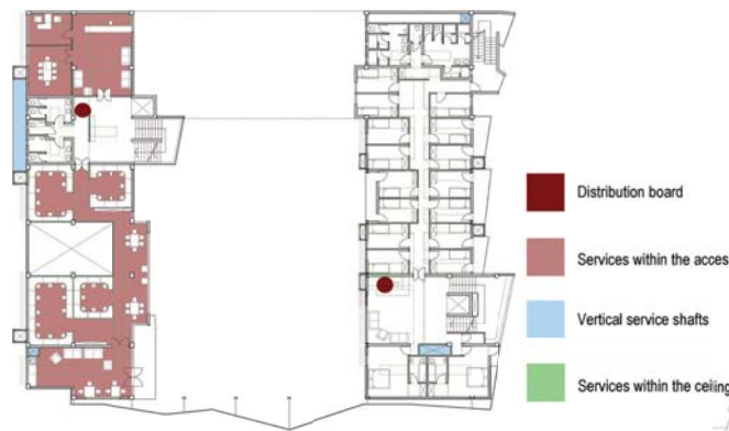
Fig. 7.37: Service distribution: fourth floor
