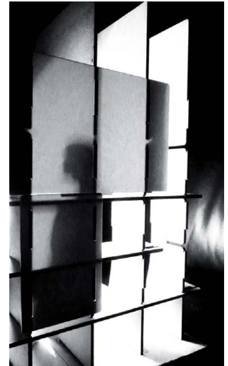
FIGURE 6.22 Shear panel prototype: Perspex
