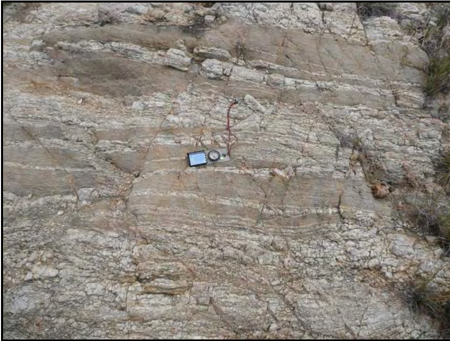
Figure 27: Slightly weathered gneiss with well-preserved joint sets.
