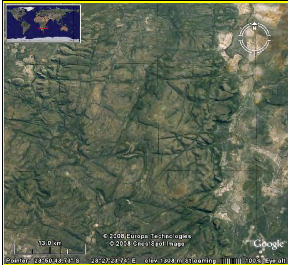
Figure 26: A Google Earth satellite image of the eastern margin of the Waterberg Group (the western boundary of the study area). Note how clearly visible the NE, E and SSE-striking joints are in the supracrustal rocks of the Waterberg and how these joints dissipate in the basement lithologies on the east.
