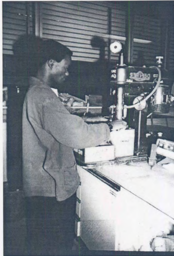
Figure 6 Operator performing rate flotation tests.
