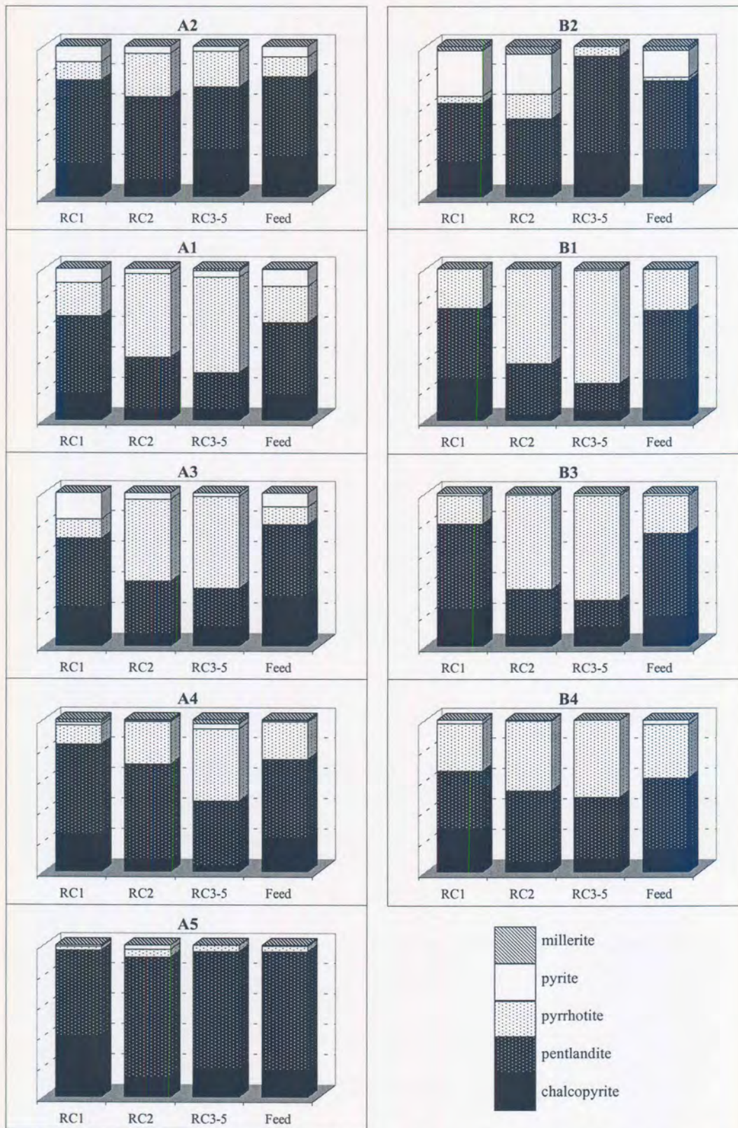
Figure 65 Relative proportions of chalcopyrite, pentlandite, pyrrhotite, pyrite and millerite in three flotation concentrates of samples from Areas A and B. RC1 = (rougher concentrate 1, 0-1 minutes), RC2 = (rougher concentrate 2, 1-3 minutes) and RC3-5 = (combined rougher concentrate 3, 4 and 5, 3-20 minutes)
