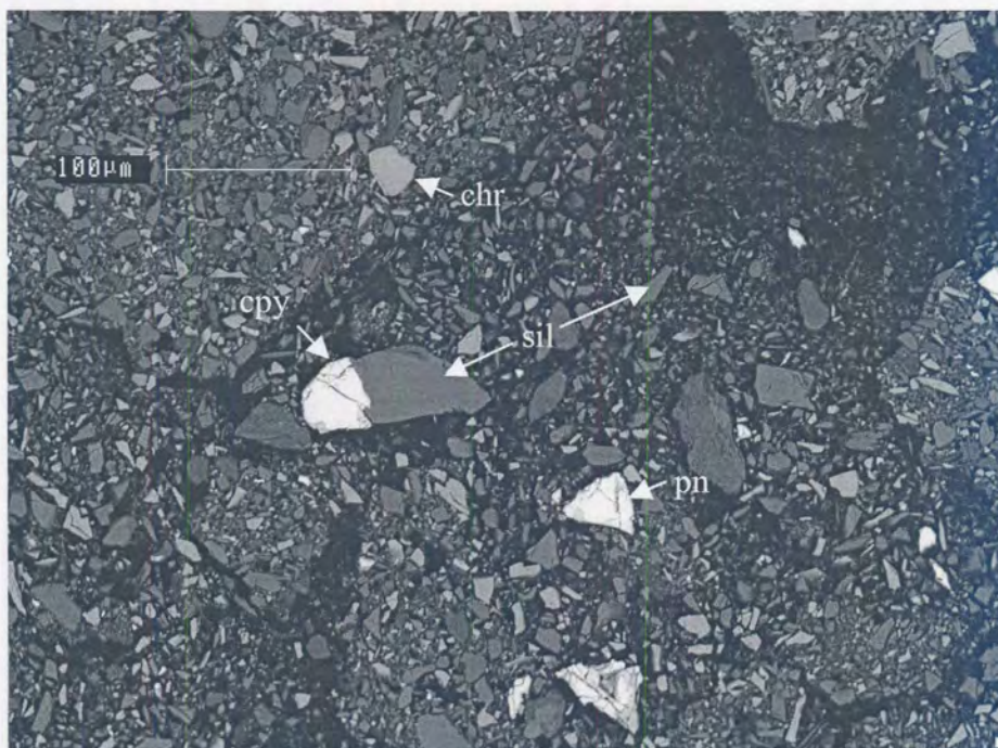
Figure 57 Backscattered-electron image of a flotation concentrate sample. The sample consists predominantly of fine-grained liberated chromite ( chr ) and silicate ( sil ). Note the coarser silicate grain forming part of a composite particle with chalcopyrite ( cpy ). A liberated pentlandite ( pn ) grain can also be seen.
