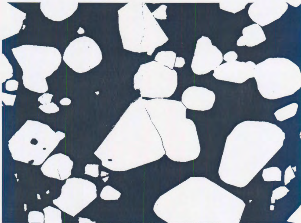
Figure 10 Binary image of chromite in Figure 9.
