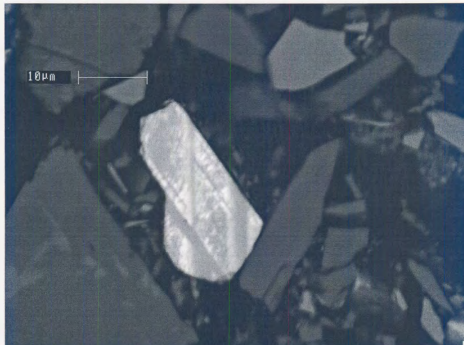
Figure 71 Liberated pentlandite grain with exsolved Pt-Rh-Cu-Ni-sulphide in flotation concentrate. Backscattered-electron image.
