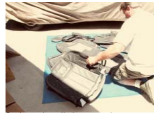
Seat panels pulled over seats
