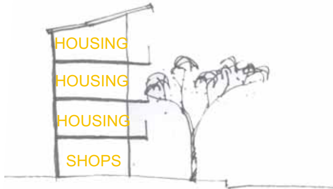
FIG 3-11: FOUR STOREY LIMIT
