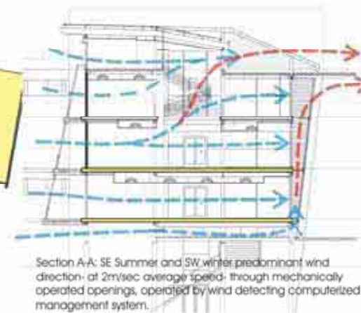
Section A-A: NE Summer and winter predominant wind direction - at 2m/sec average speed - through mechanically operated openings, operated by wind detecting computerized management system.
