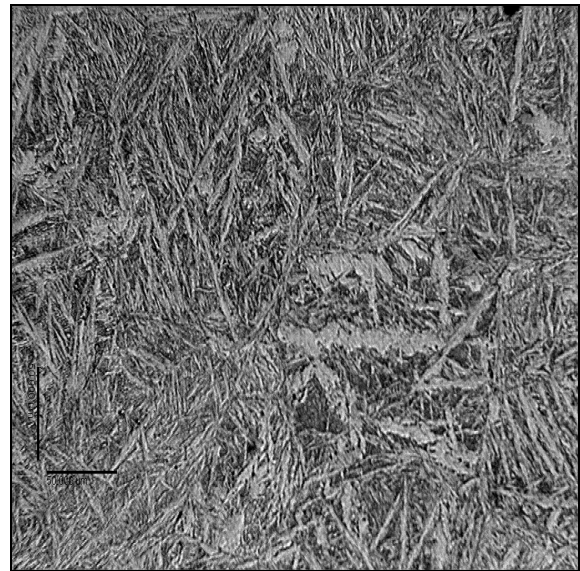
Figure D.33: Optical micrograph of HEAT 1, austenitised at 1150°C for 15 minutes, oil quenched and sub-zero treated at -196°C. The microstructure consists of retained austenite in a martensite matrix. (Hardness: 700\pm 15 HV). (Magnification: 200x).
