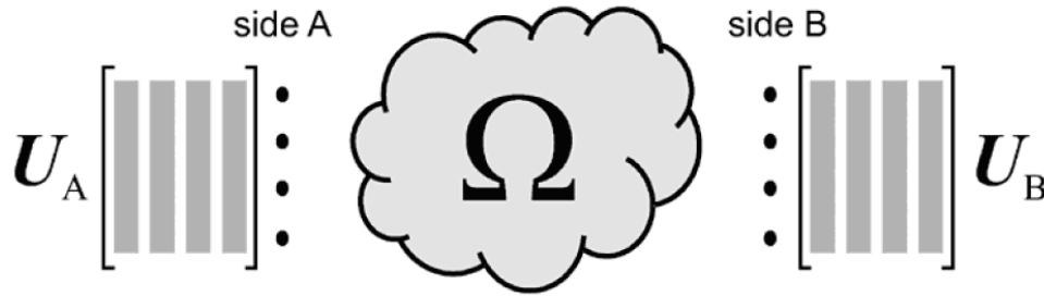
FIGURE 3.8: The parameters of the Weichselberger model as taken from [7], where A and B represent Tx and Rx respectively.
