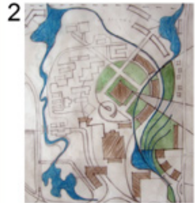
Figure 130: Masterplan attempt # 2 - storm water channels with main retention dam at lowest point of site (Author, 2008)
