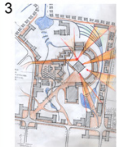
Figure 131: Masterplan attempt # 3 - move face of University to Hans Strydom Road and create portals inviting people into the campus (Author, 2008)
