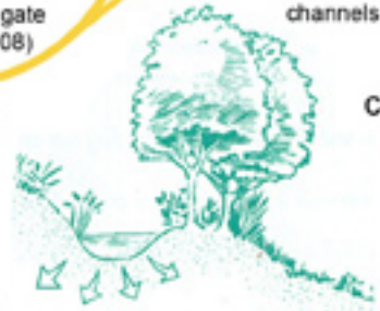
Figure 148: Water seeps into soil from irrigation channel (Nel, [S.a.]:30)
