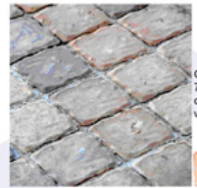
C.E.L. Paving Products: Sandstone 70mm thick cobblestone paver laid on 25mm compacted sand bed, with fine jointing sand swept and vibrated into joints.
