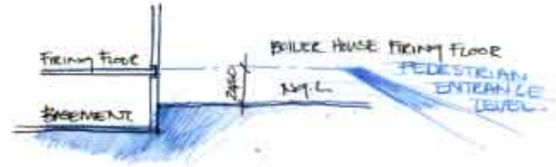
Figure D.5.5 Boiler house firing floor level
