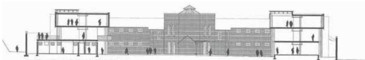
Figure 2.47: Section through new office buildings, with elevation of original building. (Source: Joubert, 2009:121)
