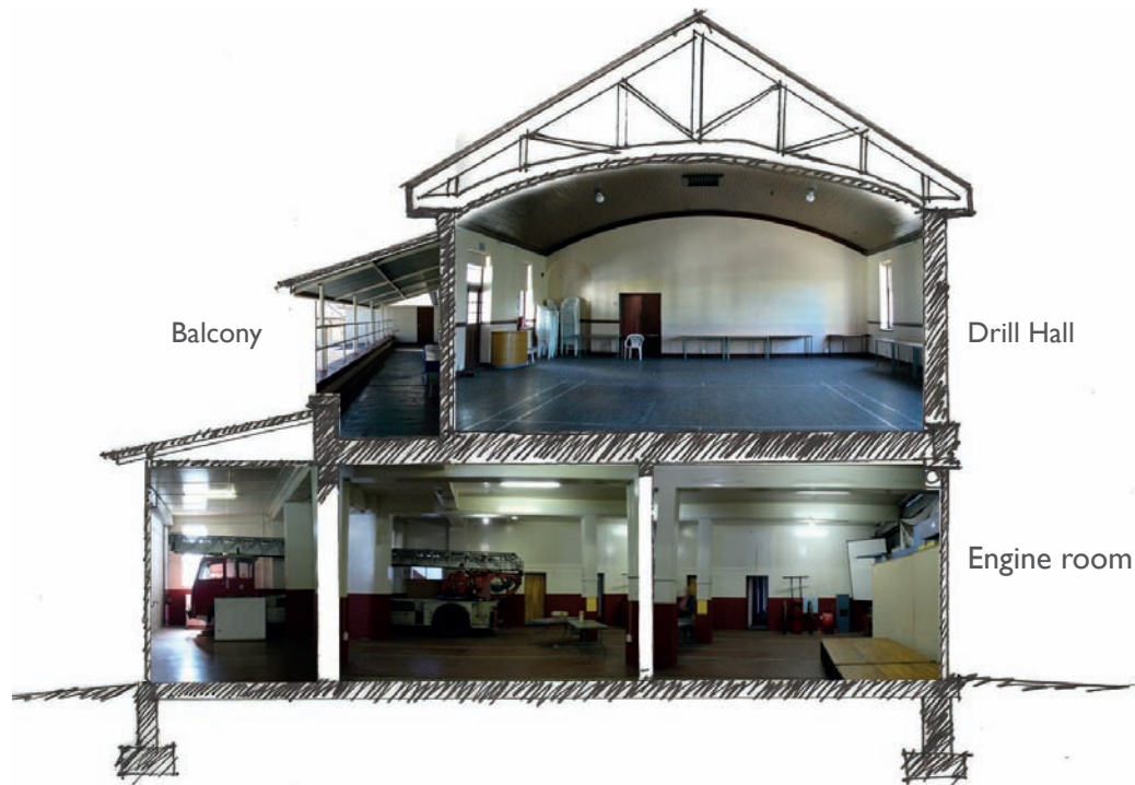
East-West section through main building
