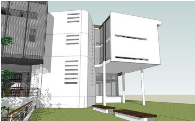
fig. 8.10_view of ablution with horizontal punctures in external envelope for solar penetration and ventilation
