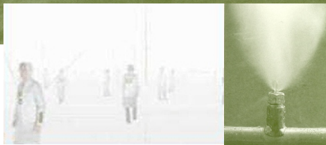
Fig 67. Nozzles used to create fog
