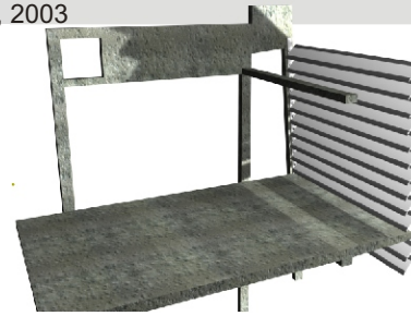
Fig. 84: Louvre position for maximum incidence
