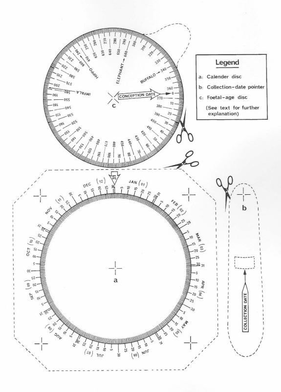
Figure 27: The three components of the device for the determination of foetal conception and birth dates from its conception age as determined by the Huggett and Widdas (1951) formula.
