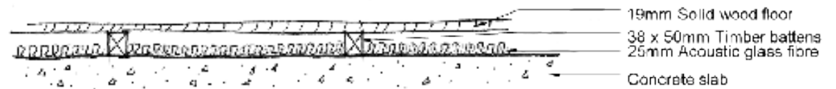
Figure 209: Section through voice booth floor.
