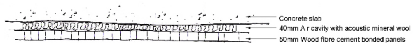
Figure 211: Section through cinema ceiling.
