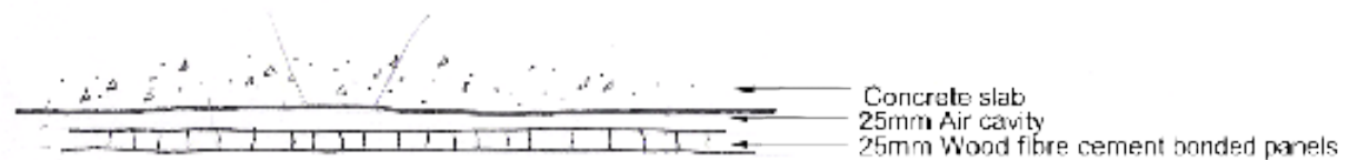
Figure 210: Section through voice booth ceiling.
