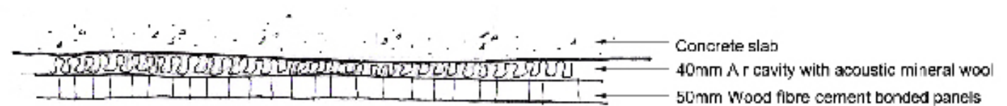
Figure 211: Section through cinema ceiling.
