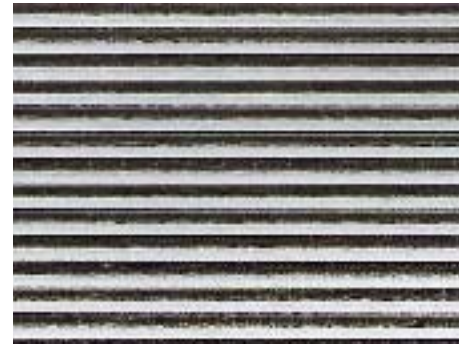
Figure 219: Ribbed sheet metal.
