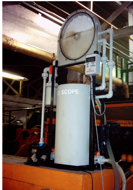
Figure 3.1. The Biofilm monitoring apparatus using refracted light.
