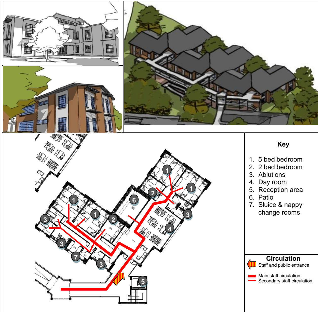
Figure 108 - Overview of the designs and layout of the first floor of the dormitories
