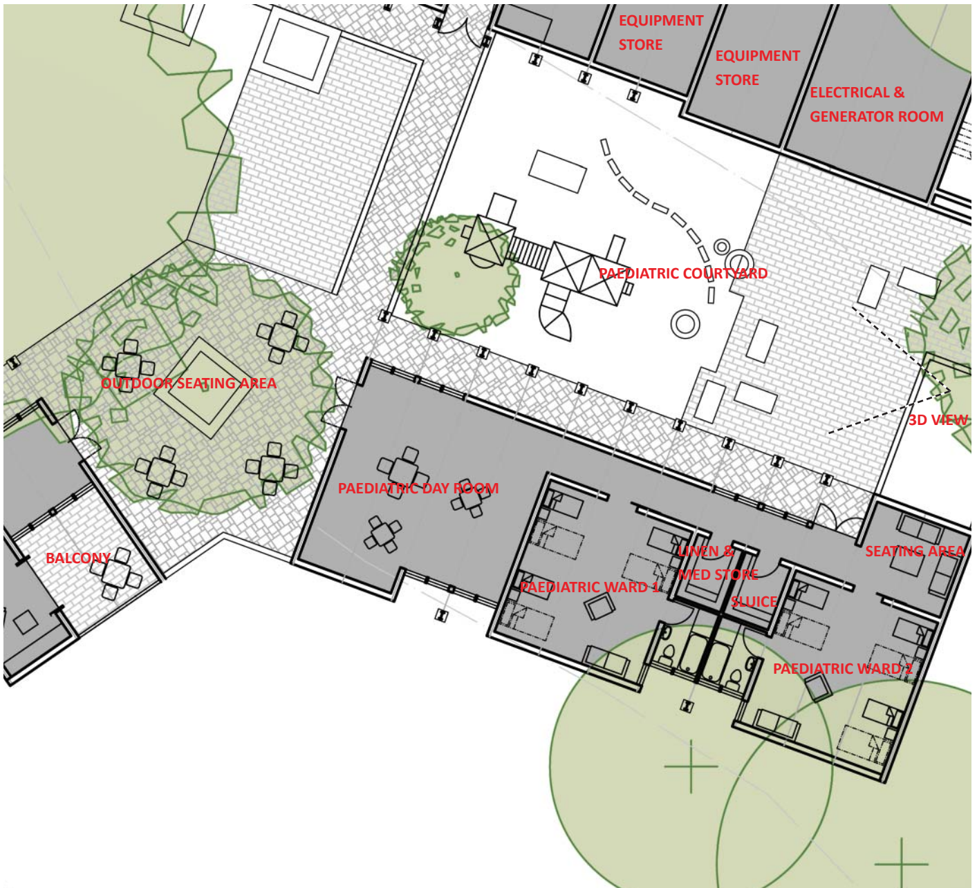
179. Ground floor plan - paediatric building
