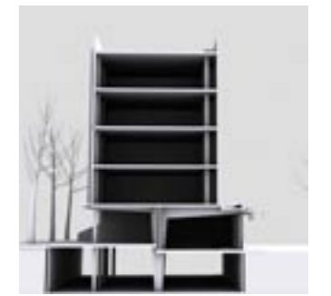
Figure 154: Section showing structural considerations for day care centre and residential block connection
