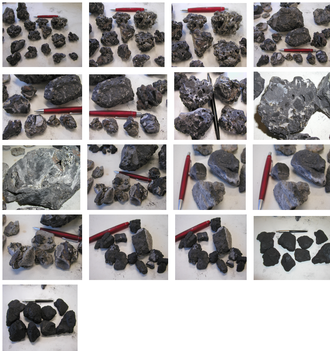
Figure: 3.8: Photographs of ash clinkers, heated rock fragments, partially burned carbon and coal particles (selected from the turn-out samples) based on their size and colour. Top row: small and medium heterogeneous clinkers with black and white colours taken from the gasification ash exiting the gasifier. Second row: small, medium and large heterogeneous clinkers with black and white colours taken from the gasification ash exiting the gasifier. Third row: large heterogeneous clinkers with black and white colours and partially burnt carbonaceous siltstone taken from the gasification ash exiting the gasifier. Fourth row: partially burnt carbonaceous siltstone, partially burnt carbonaceous shale and coal particles taken from the gasification ash exiting the gasifier and coal feedstock. Fifth row: coal particles taken from the coal feedstock.
