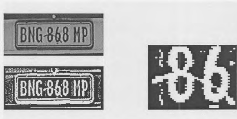
Figure 2.5: An example of a segmentation error with multiple symbols segmented as a single symbol
