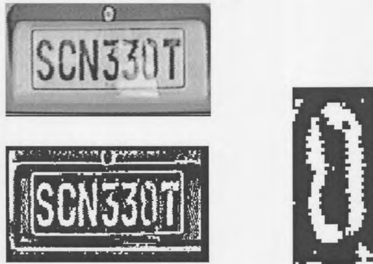
Figure 2.4: An example of a segmentation error with a broken symbol
