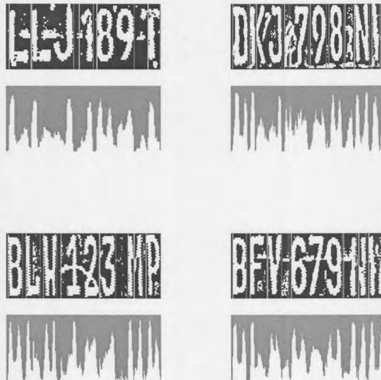
Figure 3.10: Vertical projection of licence plate images of Figure 3.8
