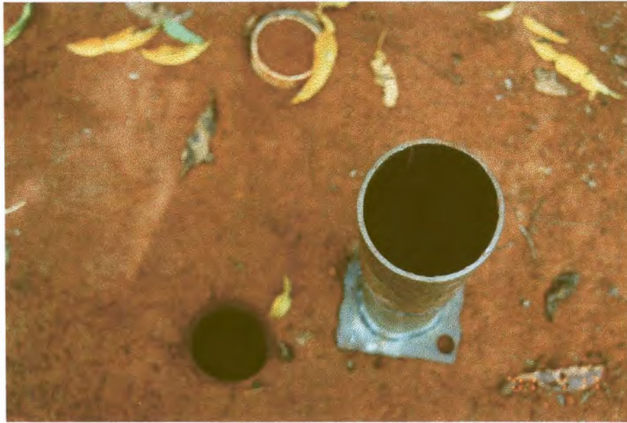
Figure 3. The lower part of the picture shows the pre-formed hole in which the micro-lysimeter is to be installed and the steel cylinder used to prepare the pre- formed hole. The upper part shows a the micro-lysimeter installed
