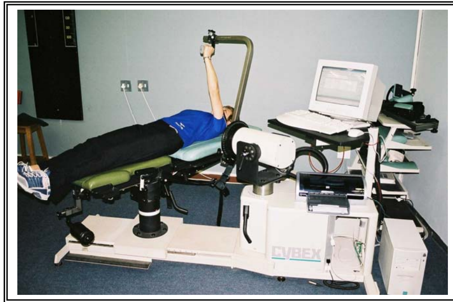
Figure 45: Isokinetic muscles strength of shoulder flexion and extension measured on the Cybex Norm.
