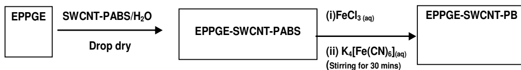
Scheme 2.3: Electrode modification procedure with Prussian blue (PB) nanoparticles.
