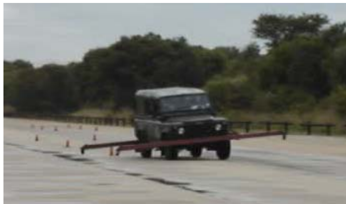
Figure 6: Land Rover with outriggers during Double lane change
