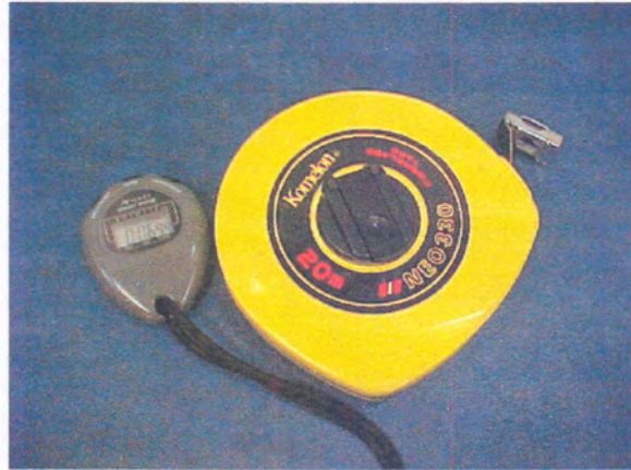
Figure 43 : Komelon NEO 330 (20 m) tape measure and Avant sport timer stop-watch
