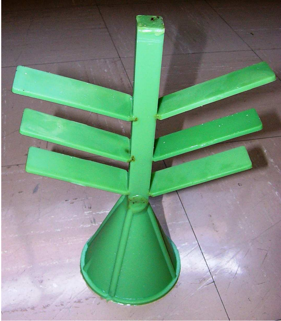
Figure 3.10: Wax pattern assembly used for investment casting (IC) of alloy A356.
