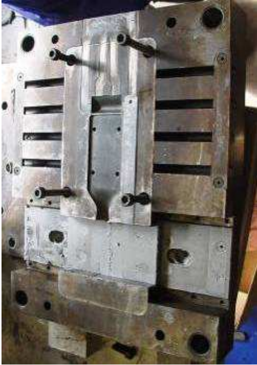
Figure 3.5: Moving half (on the left) and fixed half (on the right) of the plate die (containing the 6 \times 55 \times 100 \text{mm}^3 cavity insert) used with the LK DCC130 HPDC machine.
