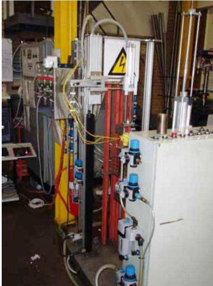
Figure 3.2: Single coil version of the CSIR rheocasting system.
