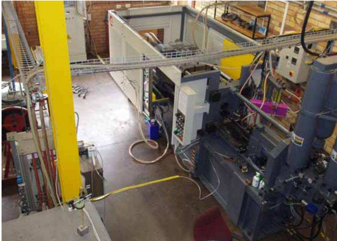
Figure 3.3: LK DCC130 shot controlled high pressure die casting machine.
