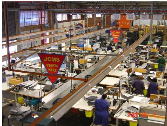
Picture 3.6 The floor layout of stand-up work stations
