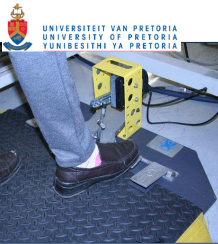
Picture 3.18 Comfortable foot wear and alternative weight bearing minimised strain on the lower limbs
