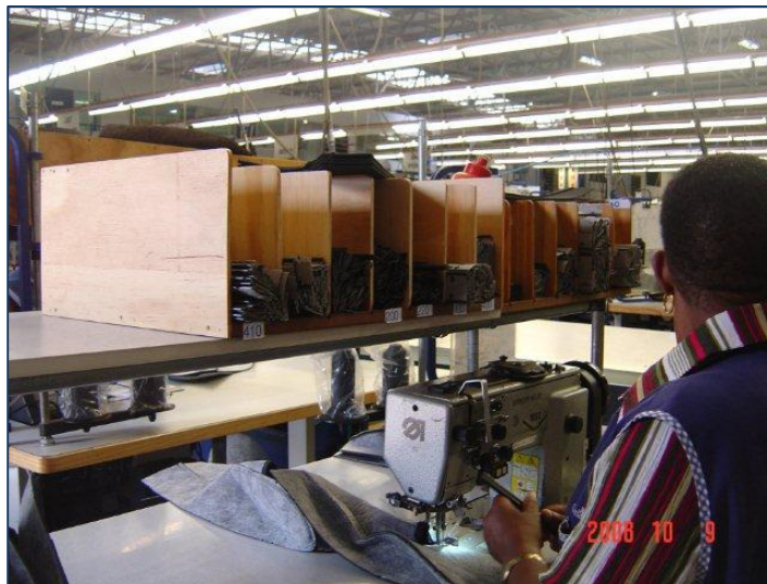
Picture 3.4 The stand-up work station demonstrates storage heights
