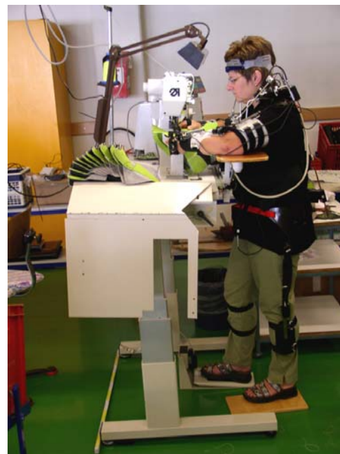
The newly developed ergonomic sewing workplace; sewing operative fitted with the CUELA measurement system
