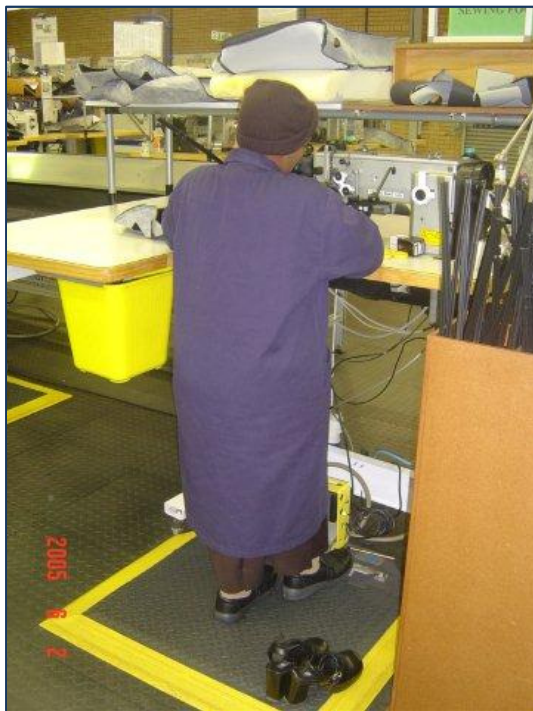
Picture 3.15 The work surface is too high, causing the sewing-machine operator to sew in shoulder abduction and - elevation
