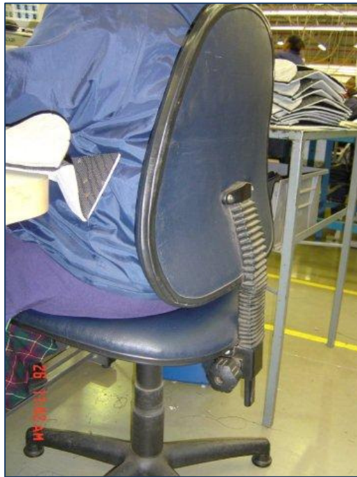
Picture 3.14 The back rest of the chair is supporting the sewing-machine operator's back
