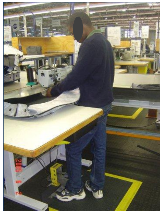
Picture 3.16 The work surface is too low, causing the sewing-machine operator to work in a forward flexed work posture
