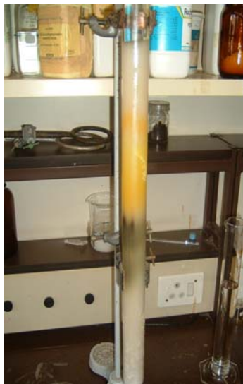
Figure 6.2. Chromatographic purification of the ethanol extract of G. africana using silica column chromatography PF 254
