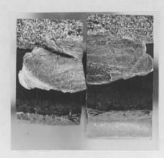
Figure 7.1: Brittle cleavage delamination fracture in a fractured 308L welded FLNFT specimen. The delamination fracture was initiated by the cleavage fracture (bright fracture surface) in the coarse grained HT HAZ.
