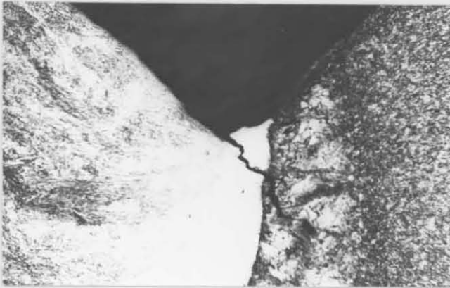
Figure 4.8: Partially fractured bead-on-plate 3CR12Ni bent specimen with the notch tip located in the weld metal. Note the short ductile crack (specimen tested at 90°C) extending from the notch tip through the weld metal into the HT HAZ (75X).
